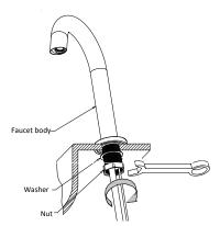
(2) Take the faucet (with flex hose and cable) and push it through the deck hole. Secure the faucet with the washer and nut.
