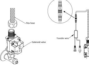
wire as illustrated. Before doing so, make sure you can see the arrows facing up and pointing at each other. Turn the medal ring in between, clockwise to
