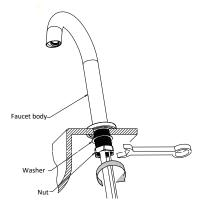
(2) Take the faucet (with flex hose and cable) and push it through the deck hole. Secure the faucet with the washer and nut.
