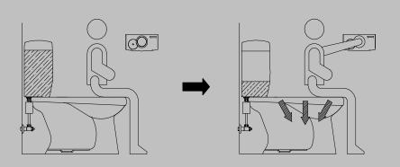
. When the user's hand approach the detection zone, the sensor sends a signal to activate the solenoid valve which lifts the flapper and flushes the toilet.
